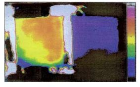
■ The right side of the specimen was coated with normal exterior paint on plain facade. The surface absorbs little energy and grows cold quickly.
